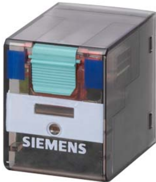
PLUG-IN RELAY, 4 CO CONTACTS, 24V DC, 6A, WIDTH 22.5MM
